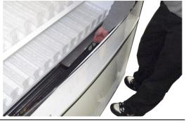
3. When refitting, ensure the return air grille and both spill trays are in place and fitted correctly. See page 9 for correct configuration.
