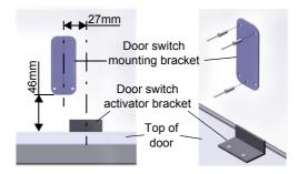
Drill two 2.5mm holes through the existing holes in the door switch bracket, and fit the door switch to the door switch bracket. Fix in place with the two 3.8 × 45 fixing screws (supplied).
