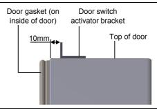
4. Fit the door switch mounting bracket above the door as pictured, drill and fix in place with three 3.2 × 8 rivets (supplied).
