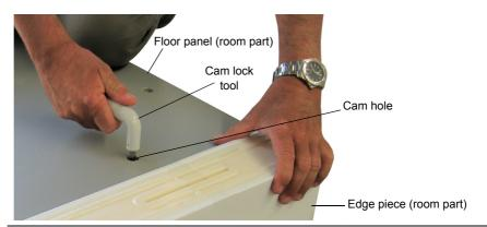
2. Rotate the tool clockwise to lock the room parts together.
