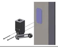
4. Remove the door switch cover by loosening the anchoring screw, and use a 2 × 1.5mm cable to connect the door switch to the refrigeration unit electronic controller. Note: Free block refrigeration units are are supplied with a door switch cable, just connect the cable to the door switch connector block.
