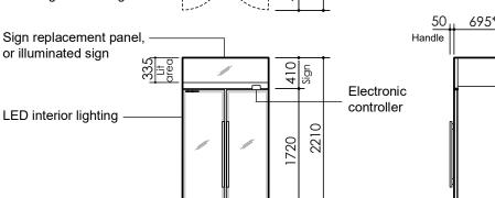
Dimensional tolerances Before installing this cabinet allow the following dimensional tolerances: Linear Overall cabinet dimensions dimensions Less than 1 metre ±5 mm More than 1 metre -5 mm to +10 mm Length of multiple cabinets At each joint At each end wall +15 mm -5 mm to +10 mm +15 mm
